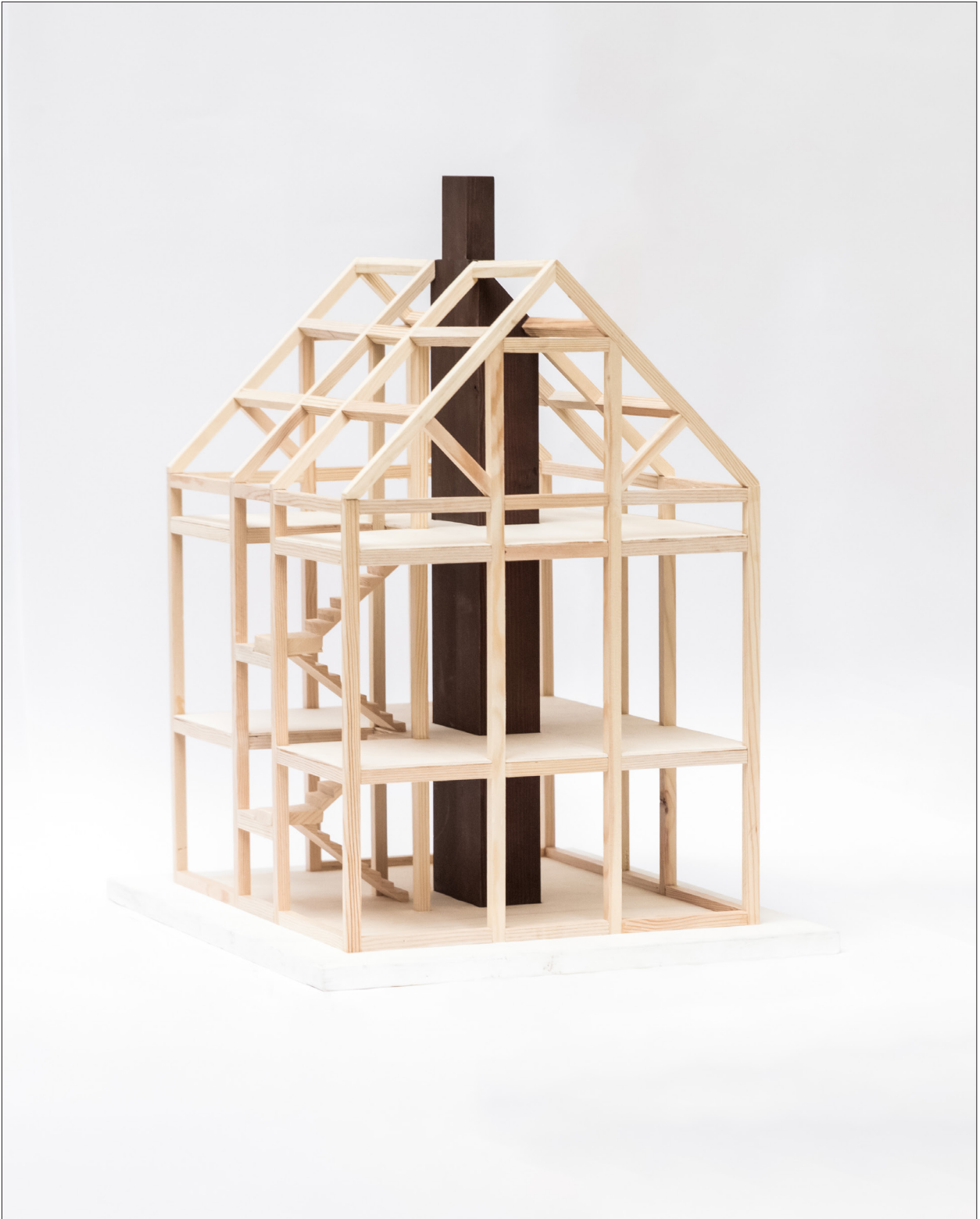
Framing model at 1:20 with masonry core in dark-brown wood.
