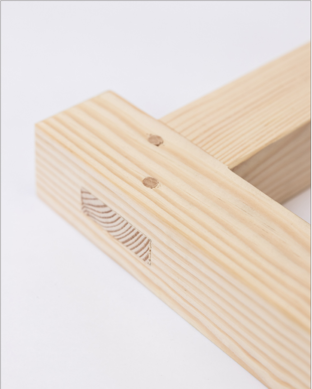
Finished mortise and tenon joint with timber.
