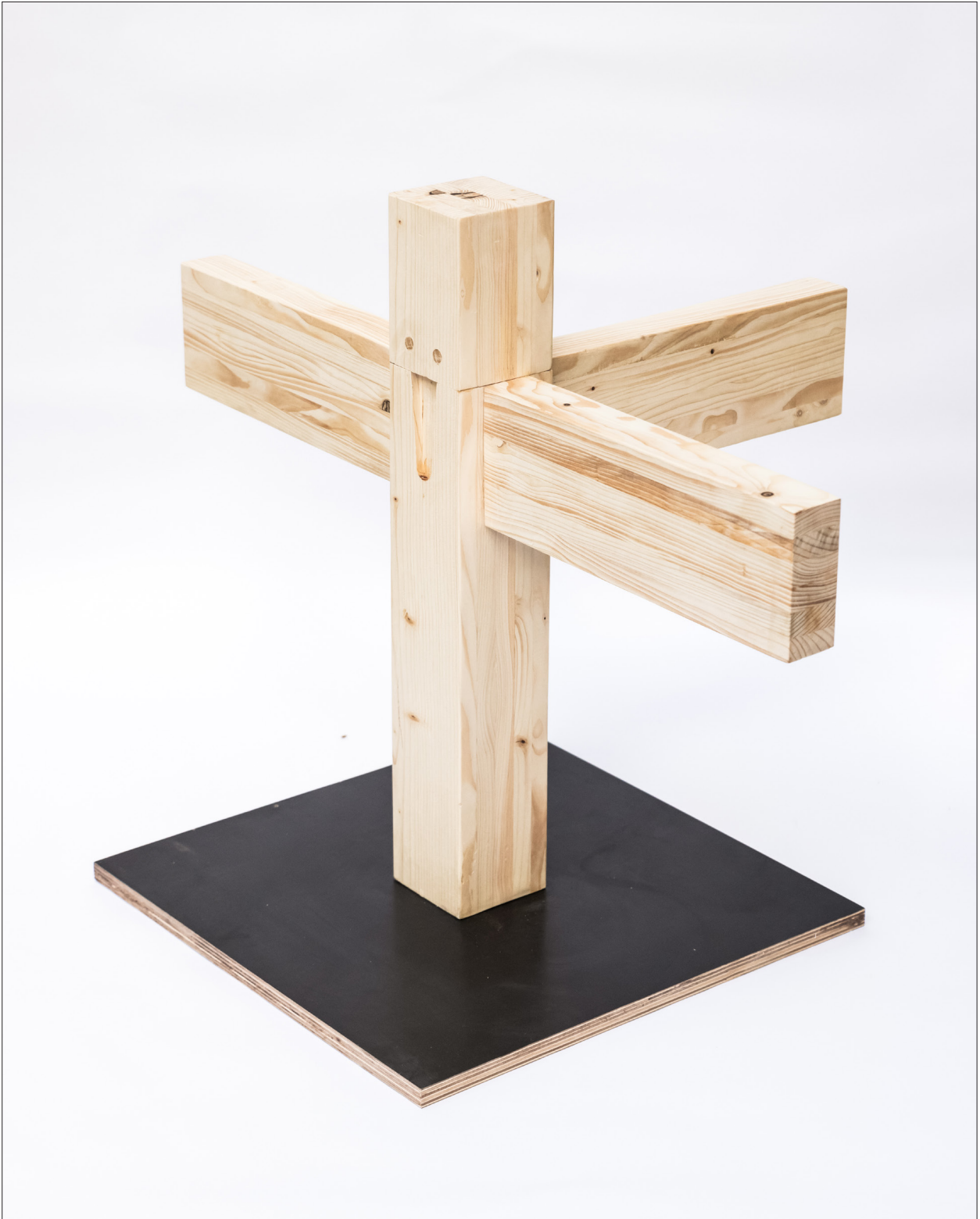
Connection model in pine at a scale of 1:2.
