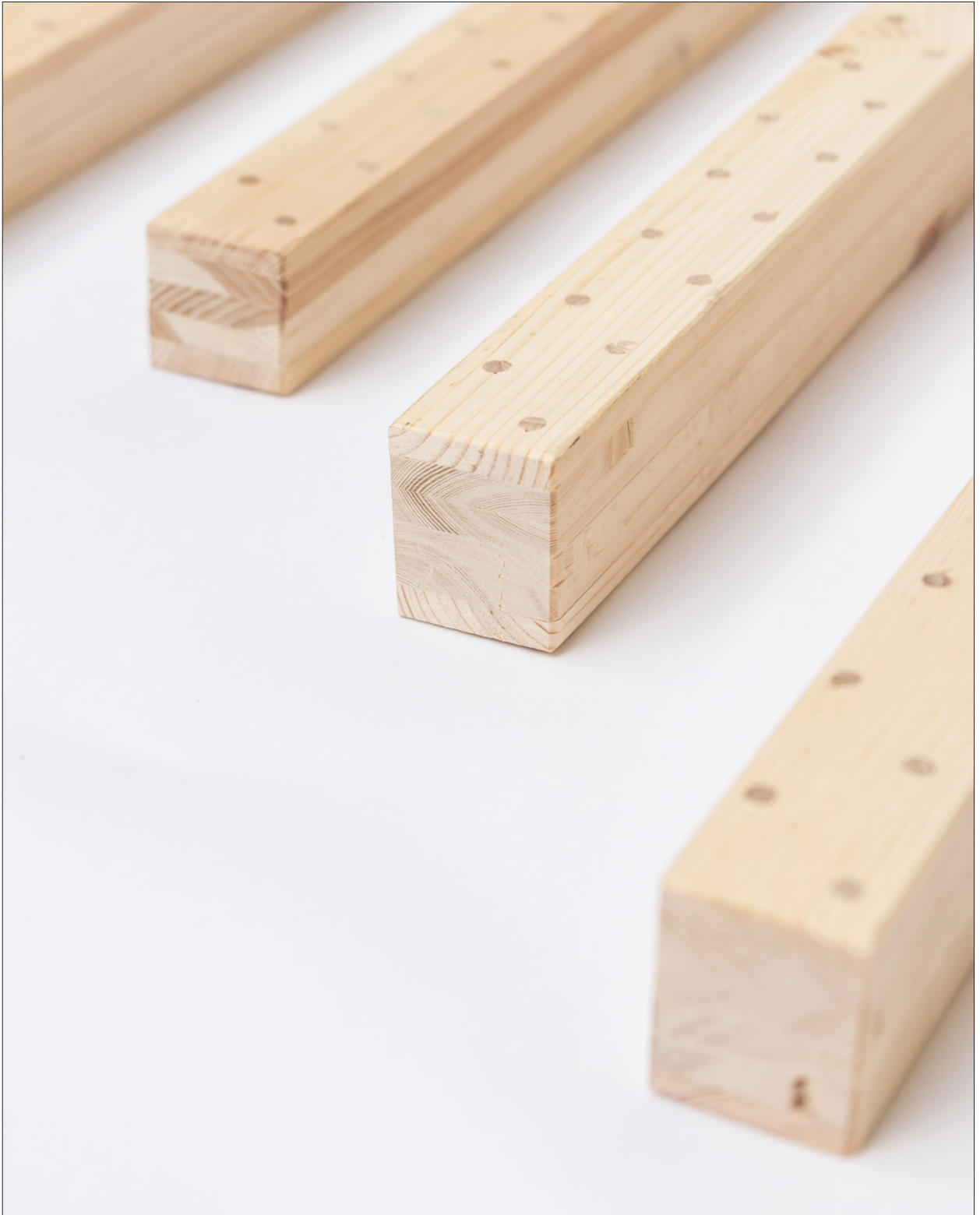
Finished Dowelam specimens.
