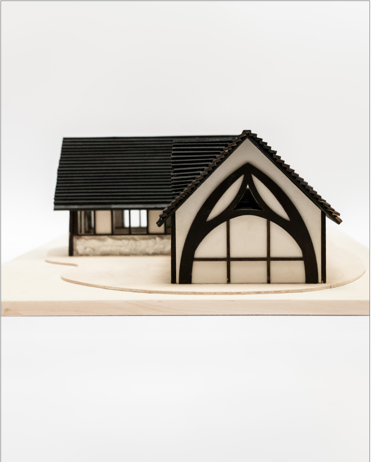
Side view of model, showing cruck-framed gable end in glulam.
