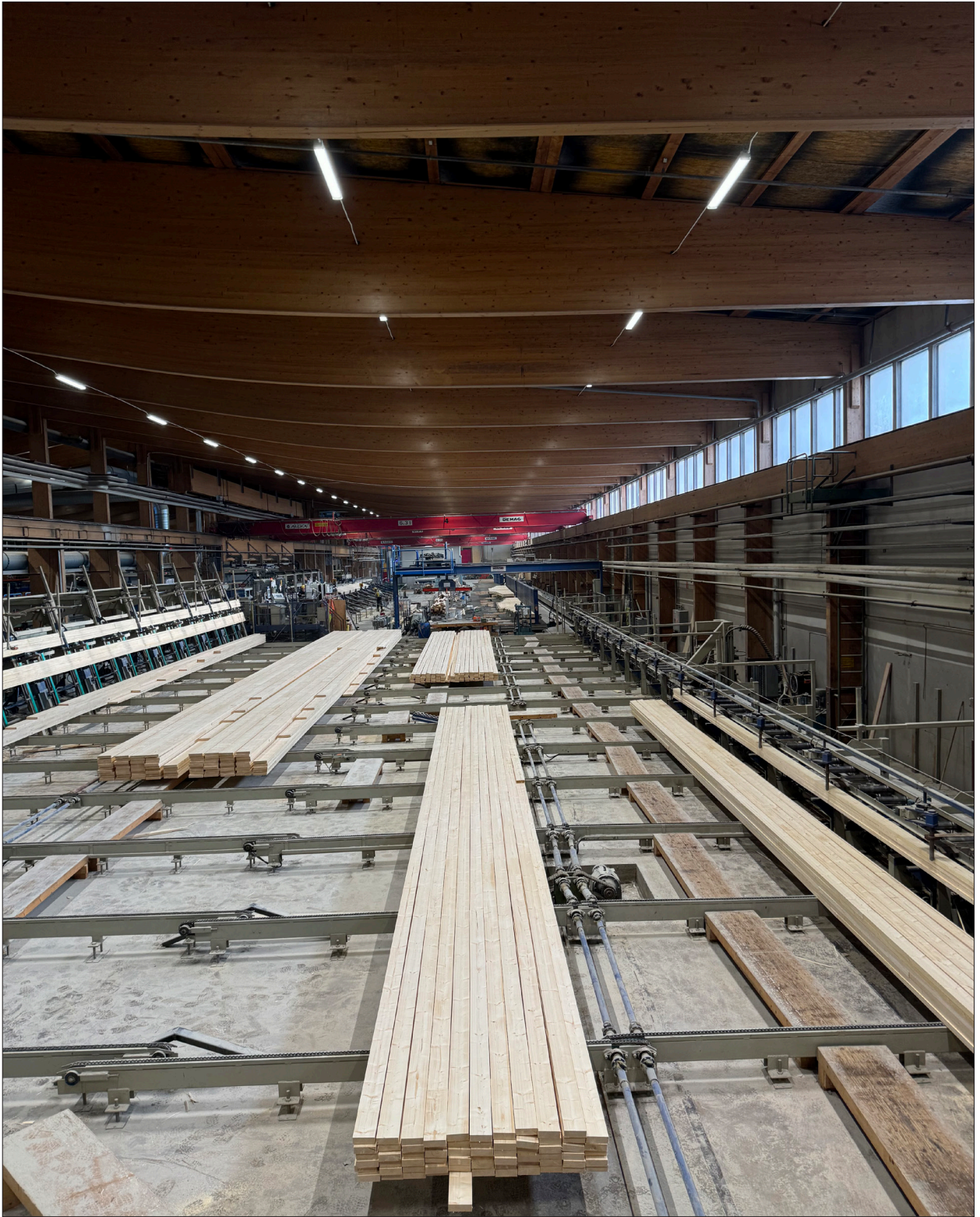
Fig. 4 Lamellas waiting to be glued up at the Versowood factory in Finland. Factory roof is made from glulam.
