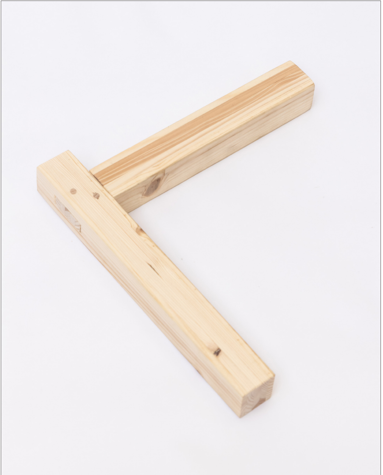
Finished mortise and tenon joint with Glulam.
