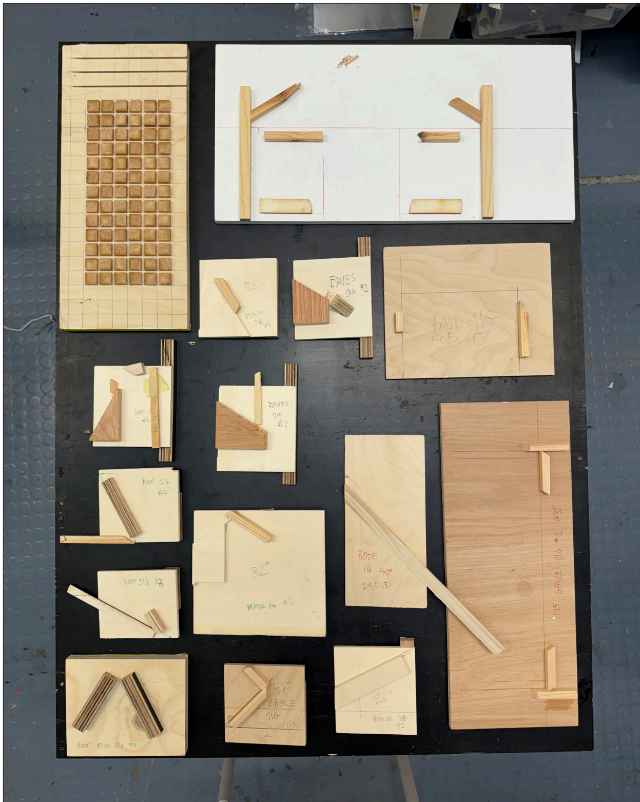
The various jigs used to make the 1:20 models. Some jigs used in assembly, most used with the bandsaw.
