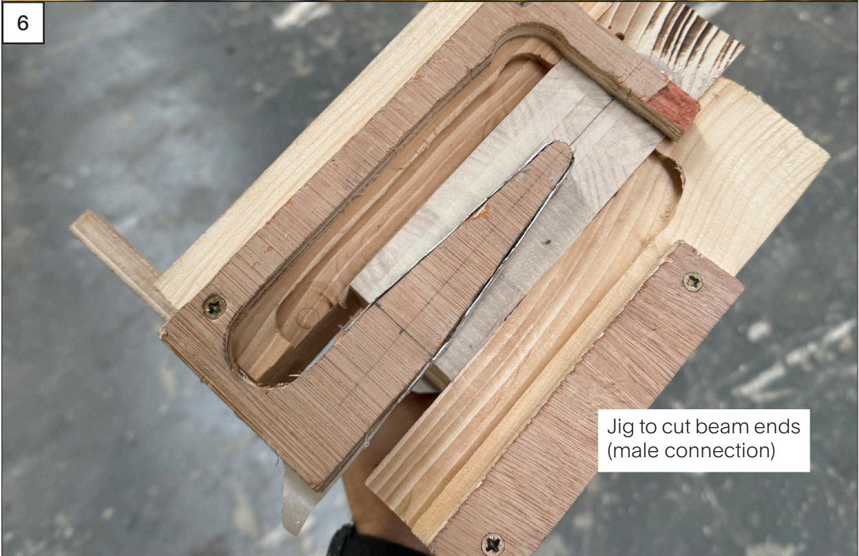
Tenon cut and chamfered
